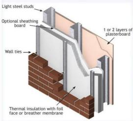
Thin sheets of galvanized steel can be formed into steel studs for use as a building material for rough-framing in commercial or residential construction, and many other applications. The dimension of the room is established with horizontal track that is anchored to the floor and ceiling to outline each room. The vertical studs are arranged in the tracks, and fastened at the top and bottom.
